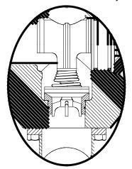
FIGURE 4-3: Valve Cage Spring Retainer
