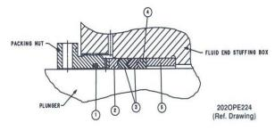
FIGURE 4-2 Packing Assembly
