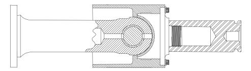
FIGURE 4-5 Crosshead Assembly
